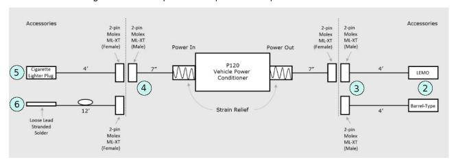
As mentioned before, there is a choice of Power Input cables terminated with either a vehicle cigarette lighter plug or two loose leads stranded solder. The Power Output cable choices depend on the equipment's power port type, LEMO or Barrel type. Use the appropriate cables for your setup.
